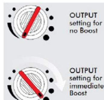
**TIP** When the next charging period starts the airflow release will close. To retain the optimum heat for a boost the next day, reset the output to minimum before the start of the next charging period which is normally overnight.
